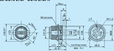
Note: Fixing nut, washer and fixing nut or fixing plate are attached as standard accessory.
